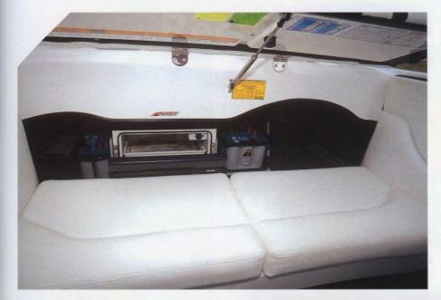
ABOVE: Under the aft lounge are two insulated coolers, whilst behind it is a fridge plus access to twin batteries, the oil container and more storage space below the aft deck.
